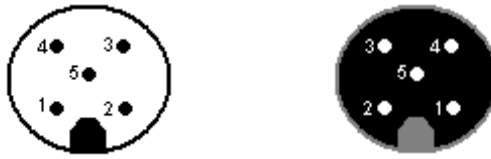
Figure 7: Pin code: Connection plug / socket for 5-pin version
