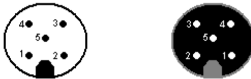
Figure 6: Pin code: Connection plug / socket for 5-pin version
