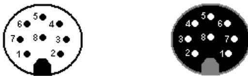
Figur 1: Pin code: Connection plug / socket for 8-pin version
