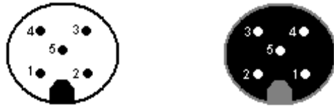
Figure 2: Pin code: Connection plug / socket for 5-pin version
