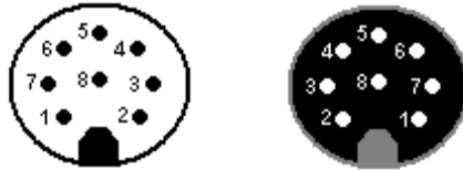
Figure 5: Pin code: Connection plug / socket for 8-pin version
