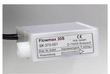
The ultrasonic flowmeter in beverage dispensing systems for alcoholic and nonalcoholic drinks. The contact-free flow measurement with no moving parts is wear and maintenance free. The free pipe cross-section over the whole channel geometry meets maximum hygienic requirements. Mechanical and / or chemical cleaning is possible without affecting the meters. Opening the beverage line and the meter can be dropped.
